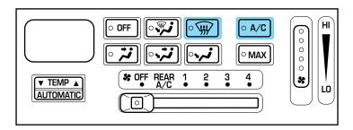
Press the [NC] (A/C) and (DEF) simultaneously for one second while rotating the fan speed dial upward until it stops moving, to switch between Fahrenheit and Celsius.
